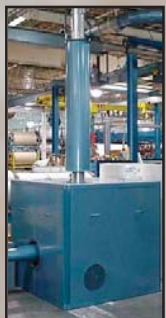
Sound attenuation devices block noise.
