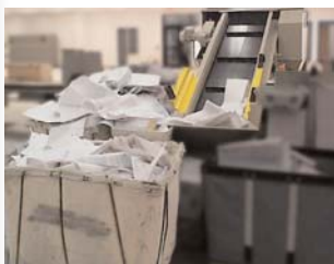
To automatically deal with large volumes of startup and other paper waste, PAC designed and provided this automated document destruction system. After loading onto the belt conveyor, the system shreds, transports and bales it with virtually no human interaction.
